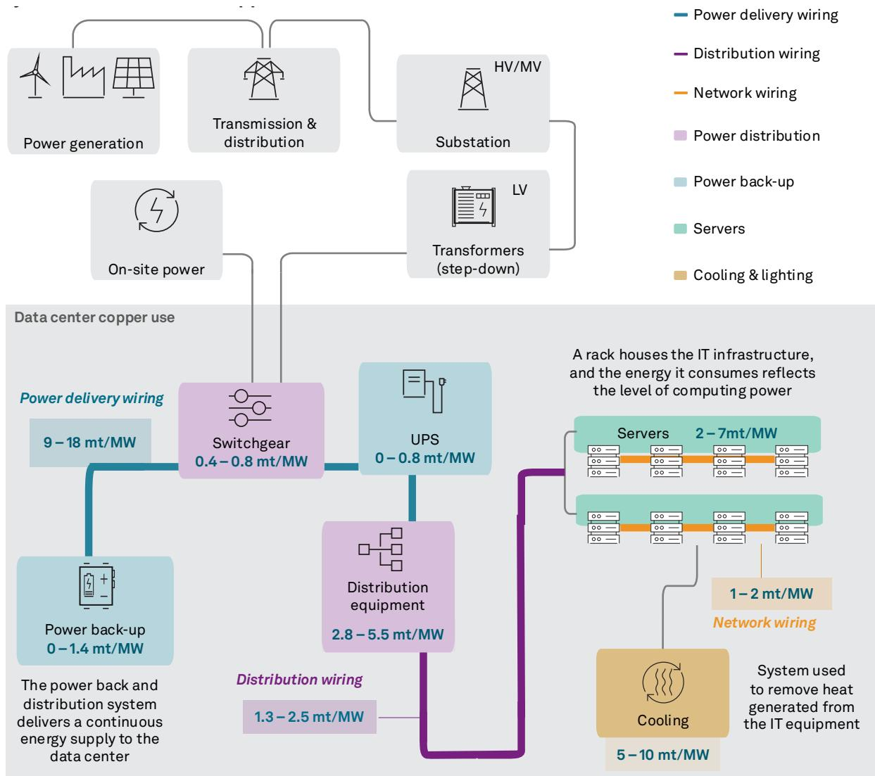
Notes: Ranges consider redundancy configurations of N, N+1 and 2N.; HV: High voltage; MV: Medium voltage; LV: Low voltage; UPS: uninterruptible power supply
